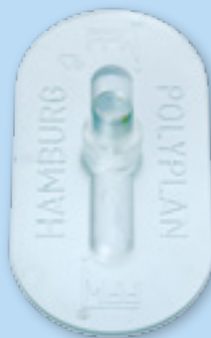
Adhesion packer oval (1131 A)< made of transparent polycarbonate, size 50 x 100 mm, outside thread M 10 x 1.0 weight circa 15 g
