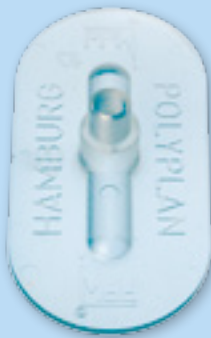
Adhesion packer oval (1131)< made of transparent polycarbonate, size 50 x 100 mm, inside thread M 8 x 1.0 weight circa 15 g
