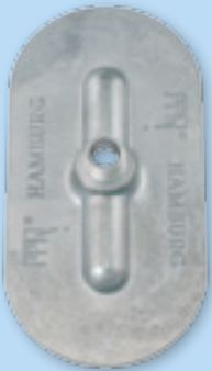
Adhesion packer oval (1130 A)< made of aluminium, size 50 x 100 mm, outside thread M 10 x 1.0 weight circa 24 g
