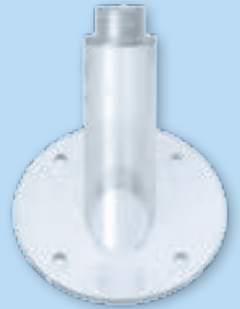
Adhesion packer round (1135)< made of transparent polycarbonate, with bevelled filler neck, inside thread M 8 x 1.0 weight circa 8 g
