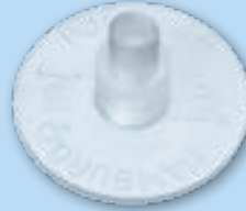
Adhesion packer round (1138 A)< made of transparent polycarbonate, 48 mm Ø, outside thread M 10 x 1.0 weight circa 7 g
