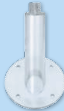
Adhesion packer round (1135 A)< made of transparent polycarbonate, with bevelled filler neck, outside thread M 10 x 1.0 weight circa 8 g
